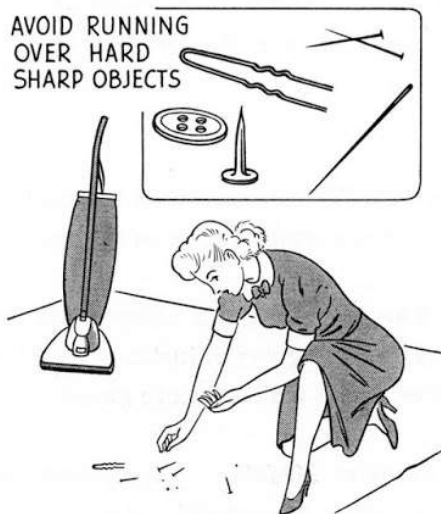
FIG. 1—Picking up pins, hairpins, tacks, pebbles or other hard objects with The Hoover may damage the belt or other moving parts
