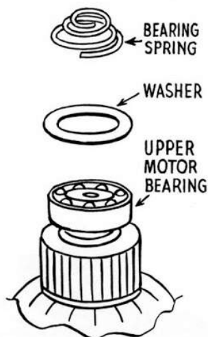
FIG. 128—Sketch of Model 425 armature, showing upper bearing assembly, including the bearing, spring and washer
