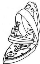
5 Lift handle and cover assembly. Remove reservoir
