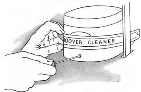
FIG. 121—Removing motor hood
