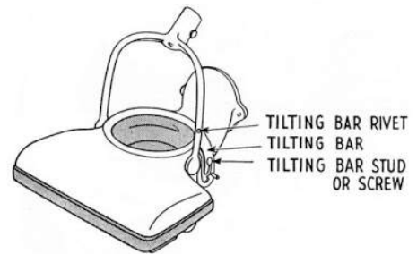
FIG. 72—Main casting with handle bail and tilting bar
