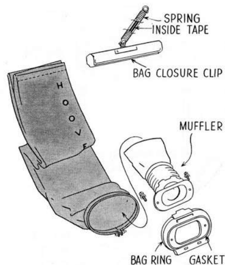
FIG. 35—The Model 60 cloth bag assembly
