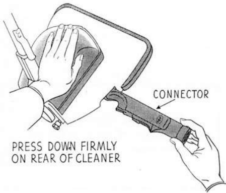
FIG. 106—Inserting connector in side of main casting
